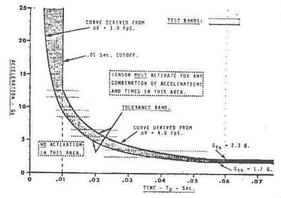
NOTE: 1. SEE SHT.1 OF 2 FOR PART NO. DESCRIPTION REMARKS ENVELOPE DIMENSIONS. BILL OF MATERIAL MATERIAL TITLE 45-3 KNICKERBOCKER AVE. △ V ACCELERATION SWITCH, 2.0G FINISH BOHEMIA, N.Y. 11716 WITH RADIAL FLEX LEADS ontrols inc. SCALE: DRAWING NO. REV DO NOT SCALE DRAWING NO. REQ'D 5/7/09 DRAWN N/A REQ'D REMOVE BURRS, BREAK SHARP EDGES. CHECKED 2014-1RFL-000 TOLERANCE UNLESS SPECIFIED: ENGINEER WEIGHT: FRACT: ±1/64 ANGLE ±0'30" DEC: .00 ± .010 APPROVED MACH FINISH: 125, APPROVED
